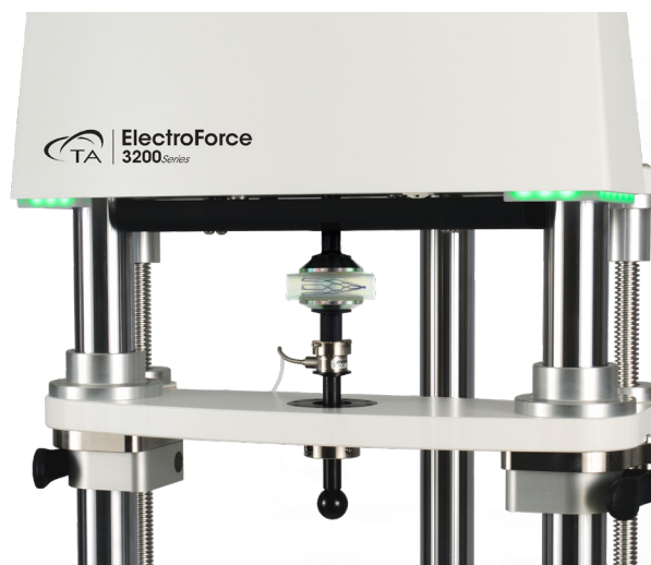
Figure 4. The ElectroForce 3200 with IVC Filter 1 Mounted for Compressive Testing
