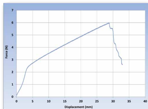
Force vs. Displacement Curve with an ElectroForce® 3200 Series III Extended Stroke Test Instrument
